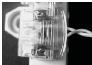
Visually inspect to ensure wire is inserted fully.
